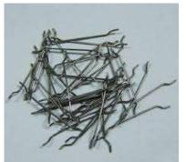
manufactured steel. Their inclusion in the concrete improves the mechanical properties of concrete significantly. As the most common matrix, which is now in use in construction industry is reinforced cement concrete.
